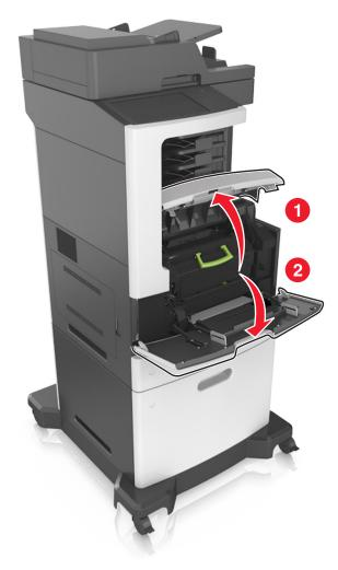
**2** Lift the green handle, and then pull out the toner cartridge from the printer.
