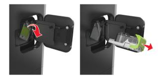
**4** Use the metal tab to lift the staple guard, and then remove any loose staples.
