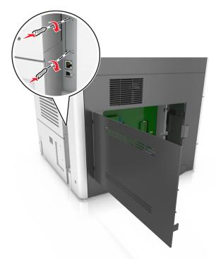
**10** Tighten the thumbscrew that is attached to the ISP.
