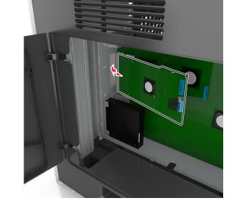
**Note:** Hold the ISP at an angle over the plastic bracket so that any overhanging connectors will pass through the ISP opening in the cage.
