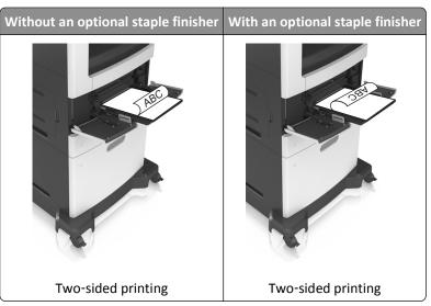
• If you are loading prepunched paper for use with the staple finisher, then make sure the holes on the long edge of the paper are on the right side of the tray.
