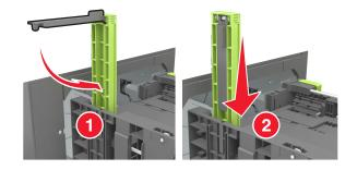
**d** Squeeze the length guide and slide it to the correct position for the size of the paper being loaded until it *clicks* into place.
