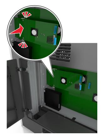
7 Lower the ISP toward the plastic bracket until the ISP is seated between the guides of the plastic bracket.
