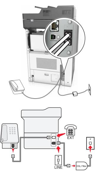
A Digital Subscriber Line splits your regular telephone line into two channels: voice and Internet. Telephone and fax signals travel through the voice channel, and Internet signals pass through the other channel. This way, you can use the same line for analog voice calls (including faxes) and digital Internet access.
