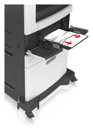
2 Flex the sheets back and forth to loosen them, and then fan them. Do not fold or crease the paper. Straighten the edges on a level surface.
