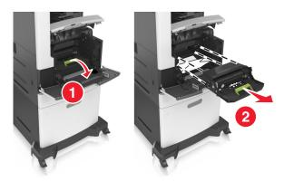
**5** Place the imaging unit aside on a flat, smooth surface.
