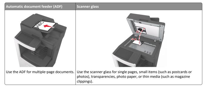
The scanner lets you scan documents directly to a computer or a flash drive. The computer does not have to be directly connected to the printer for you to receive scan to computer images. You can scan the document back to the computer over the network by creating a scan profile on the computer and then downloading the profile to the printer.
