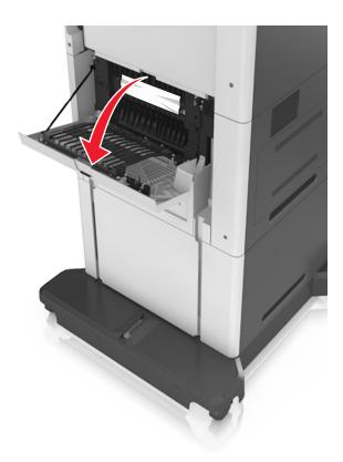
2 Firmly grasp the jammed paper on each side, and then gently pull it out.Note: Make sure all paper fragments are removed.
