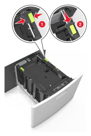
**c** Remove the A5 length guide from its holder.
