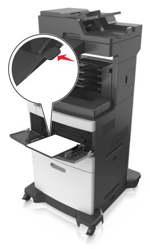
Warning—Potential Damage: Overfilling the feeder can cause paper jams.
