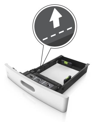
**6** For custom- or Universal-size paper, adjust the paper guides to lightly touch the sides of the stack, and then lock the length guide.
