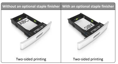
• If you are loading prepunched paper for use with the staple finisher, then make sure the holes on the long edge of the paper are on the right side of the tray.
