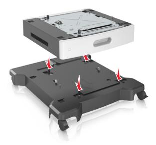
8 Align the printer with the tray, and then slowly lower the printer into place.Note: Optional trays lock together when stacked.
