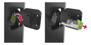
**3** Squeeze both sides of the empty staple case with your fingers, and then remove the staple case from the cartridge.
