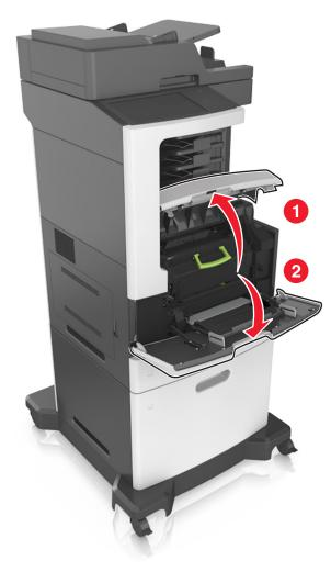
**2** Pull the cartridge out of the printer using the handle.
