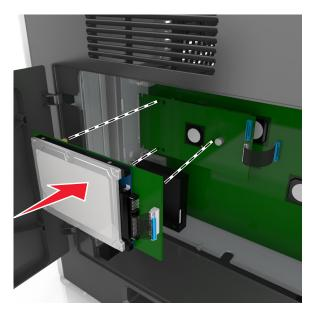
**c** Insert the plug of the printer hard disk interface cable into the receptacle of the ISP. **Note:** The plugs and receptacles are color-coded.
