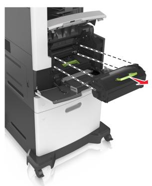
**3** Lift the green handle, and then pull out the imaging unit from the printer.
