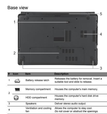
**Note**: For models with an AMD processor and a single memory module: If you replace the memory module, the new module <u>must</u> go into the same slot occupied by the module that was removed.
