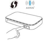
Press the WPS or AOSS<sup>™</sup> button on your wireless LAN access point/router.
