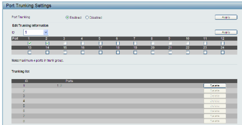
Figure 158- L2 Features &gt; Port Trunking Settings
