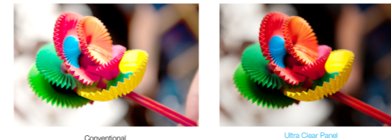
Figure 8. The Ultra Clear Panel reduces light scatter and provides clearer, more detailed images.
