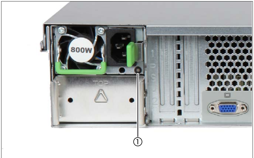
Figure 10: Indicator on hot-plug power supply unit
